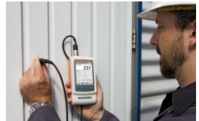
Measurement of paint coating thickness
